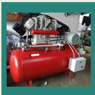
Industrial Air Compressor
